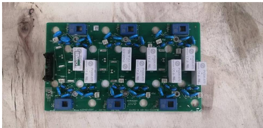
Figure 20. Front view of DC-EMI board
