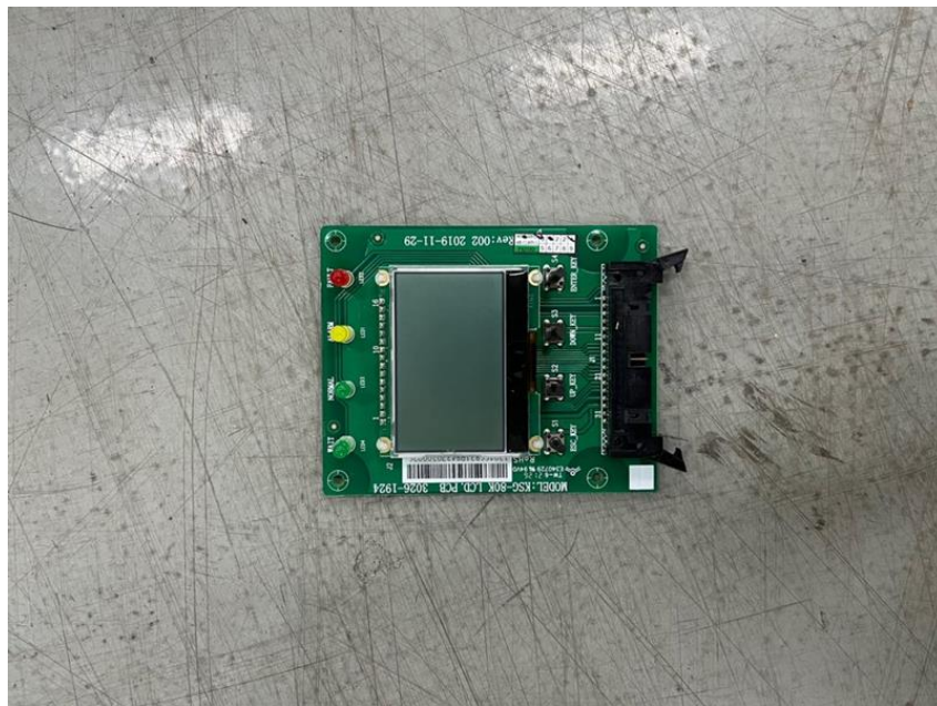
Figure 16. Front view of LCD board
